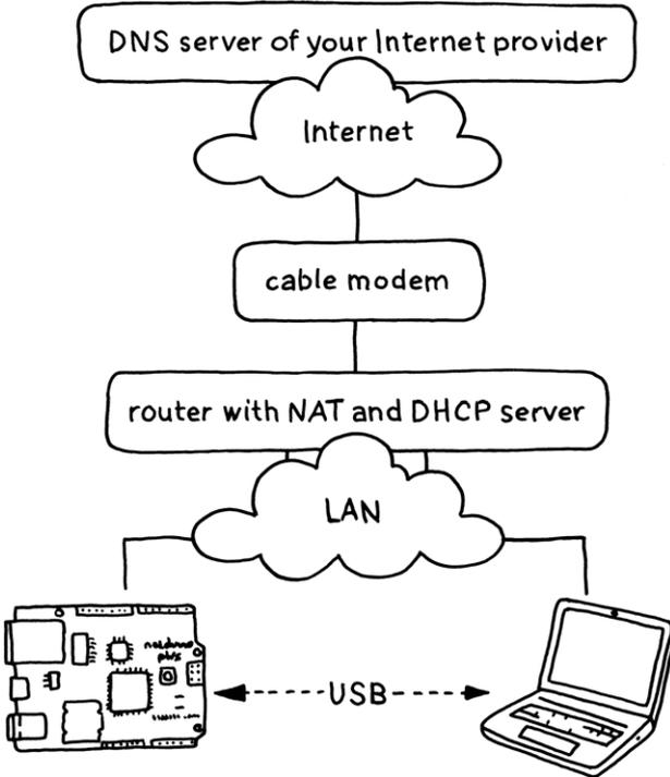
Figure 6-2. Connection of board to the Internet
